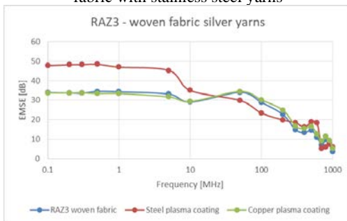
Fig. 2 - Steel and Copper plasma coating on woven fabric with silver yarns
